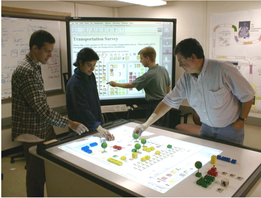
Figure 6.4: The initial version of the EDC using Smart Boards. Integrating Smart Boards for the action and reflection spaces with overhead and rear-view projection and utilizing AgentSheets to support interactivity in the action space of the Lego Blocks as the language of objects.
