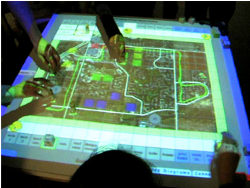
Figure 6.11: Stakeholders around the PitA-Board. Participants can interact with action space through the physical pieces, which represent objects in the simulation or can be used to perform actions using programmed border squares along the edges.
