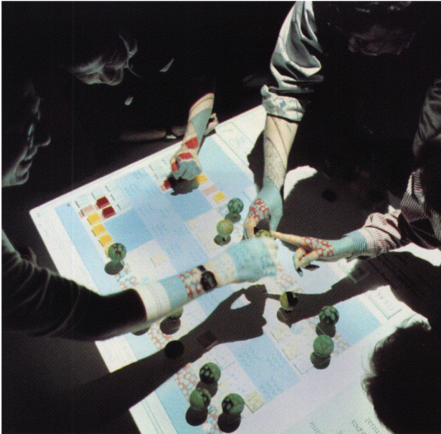
Figure 6.3: The Intersim “Wizard-of-Oz” setup. Utilizing an initial version of AgentSheets and top-down projection.
