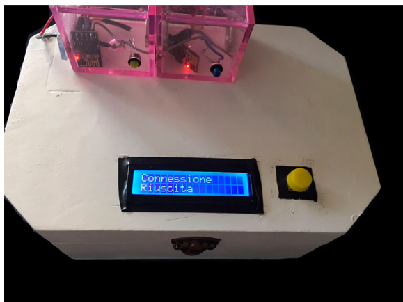
Figure 11. The pill dispenser prototype with modular pill boxes.
